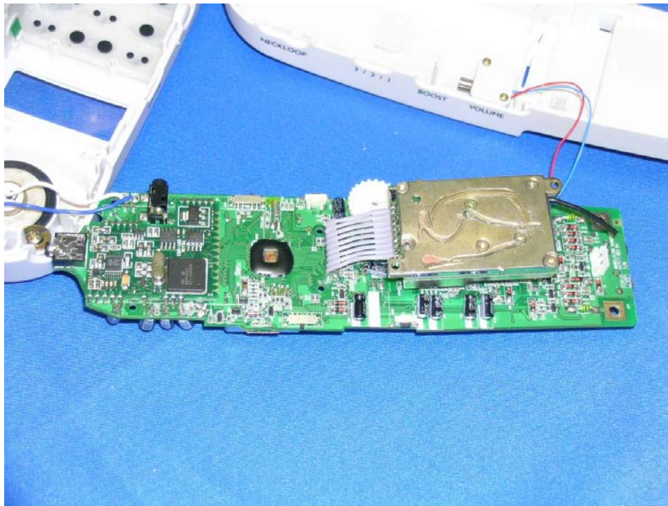
Handset Main PCB comp side (View 2)
