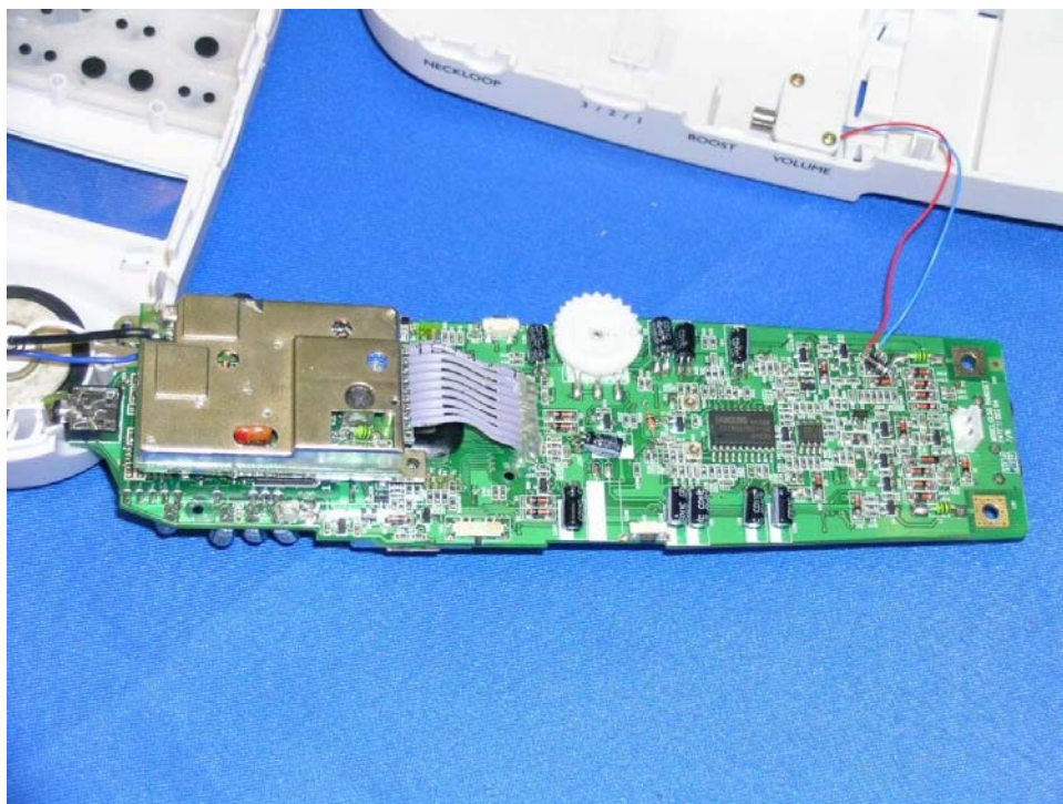
Handset Main PCB comp side (View 1)
