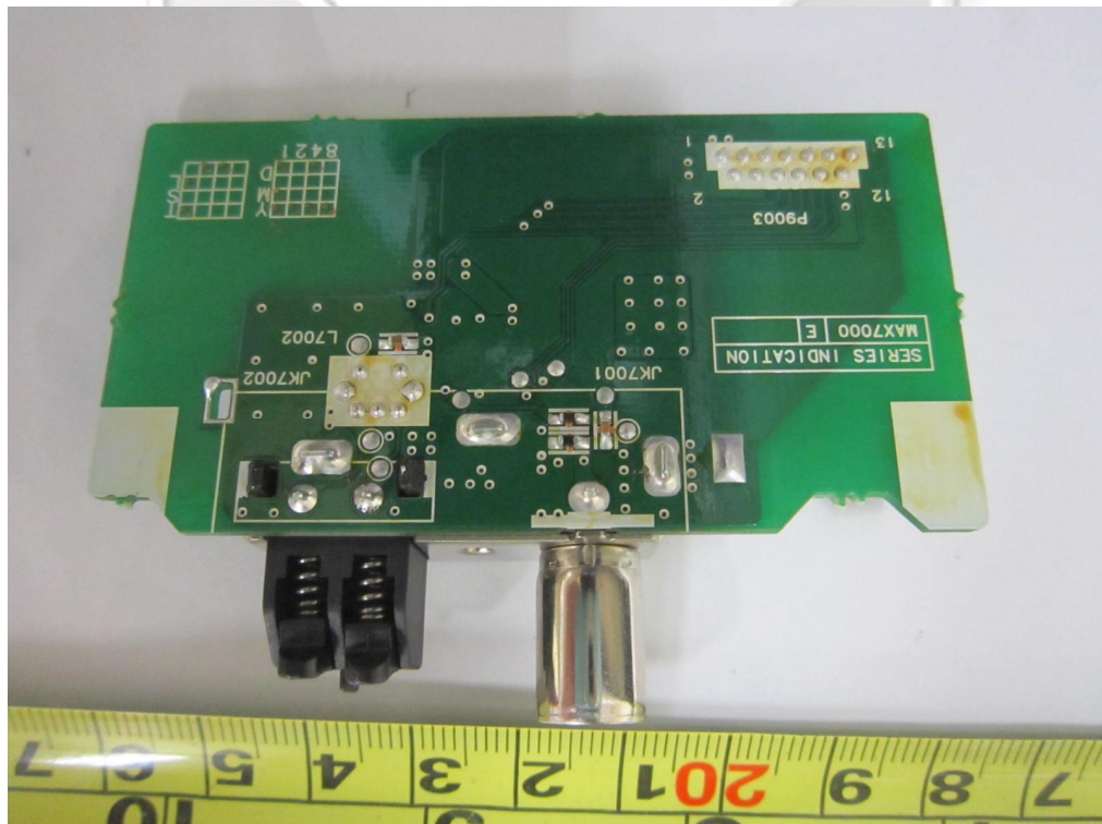
FM/AM Antenna Board PCB Trace Side
