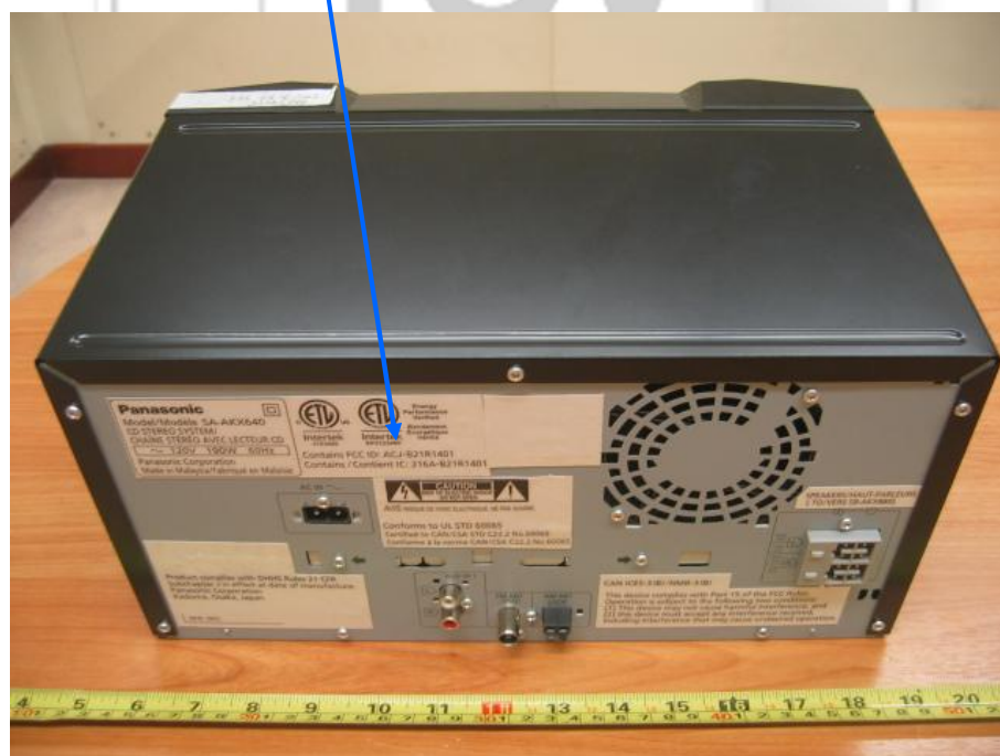
Physical Location of FCC Label on EUT
