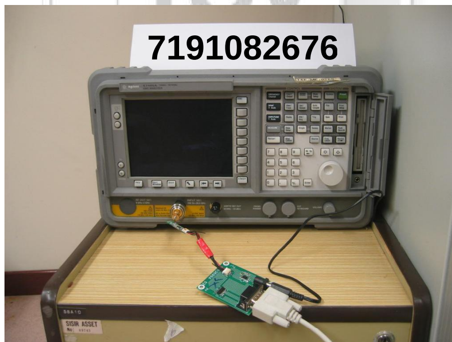
Average Frequency Dwell Time Test Setup
