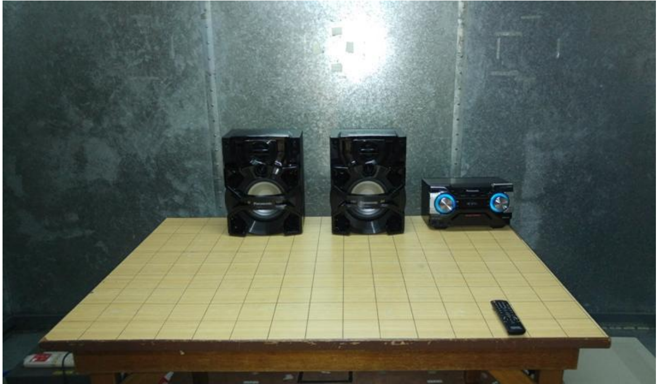
Conducted Emissions Test Setup (Front View)
