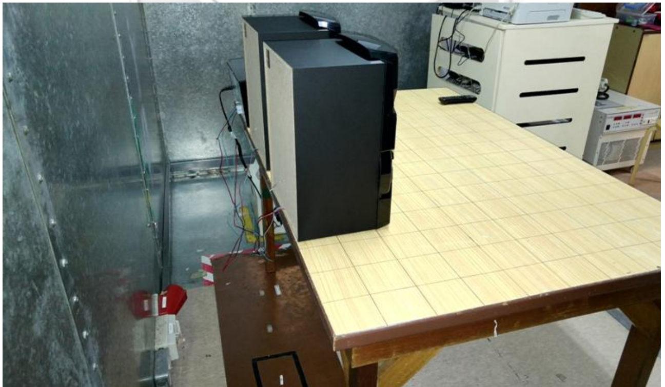
Conducted Emissions Test Setup (Rear View)
