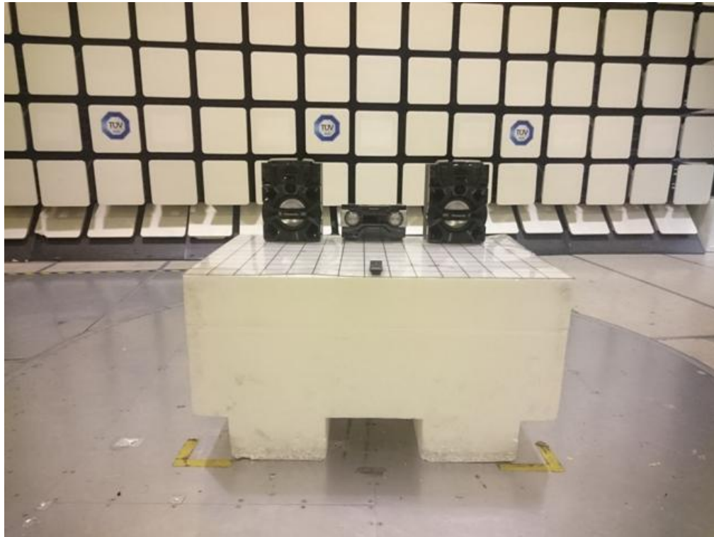
Radiated Emissions Test Setup (Front View)
