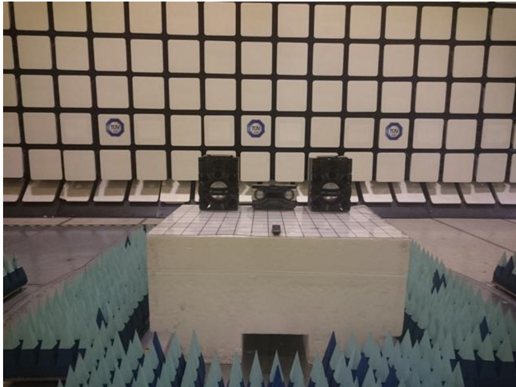
Radiated Emissions Test Setup (Front View)
