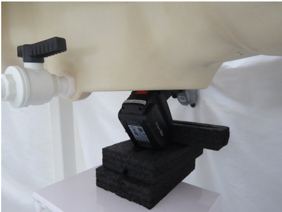
Picture 2: Back Side2, the distance from EUT to the bottom of the Phantom is 0mm
