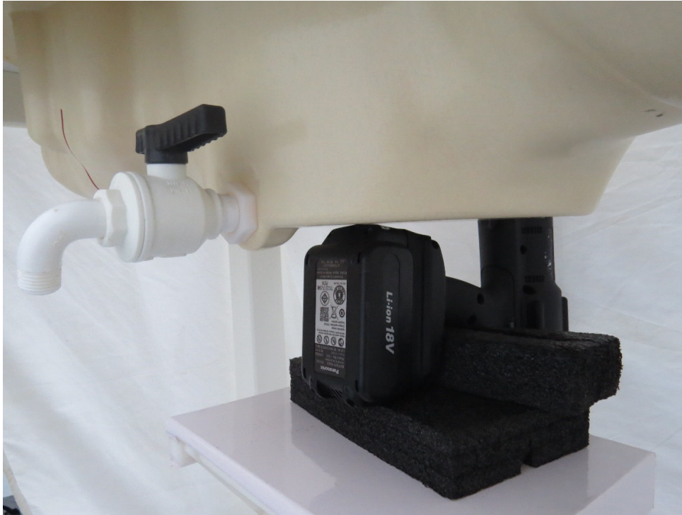
Picture 1: Back Side, the distance from EUT to the bottom of the Phantom is 0mm
