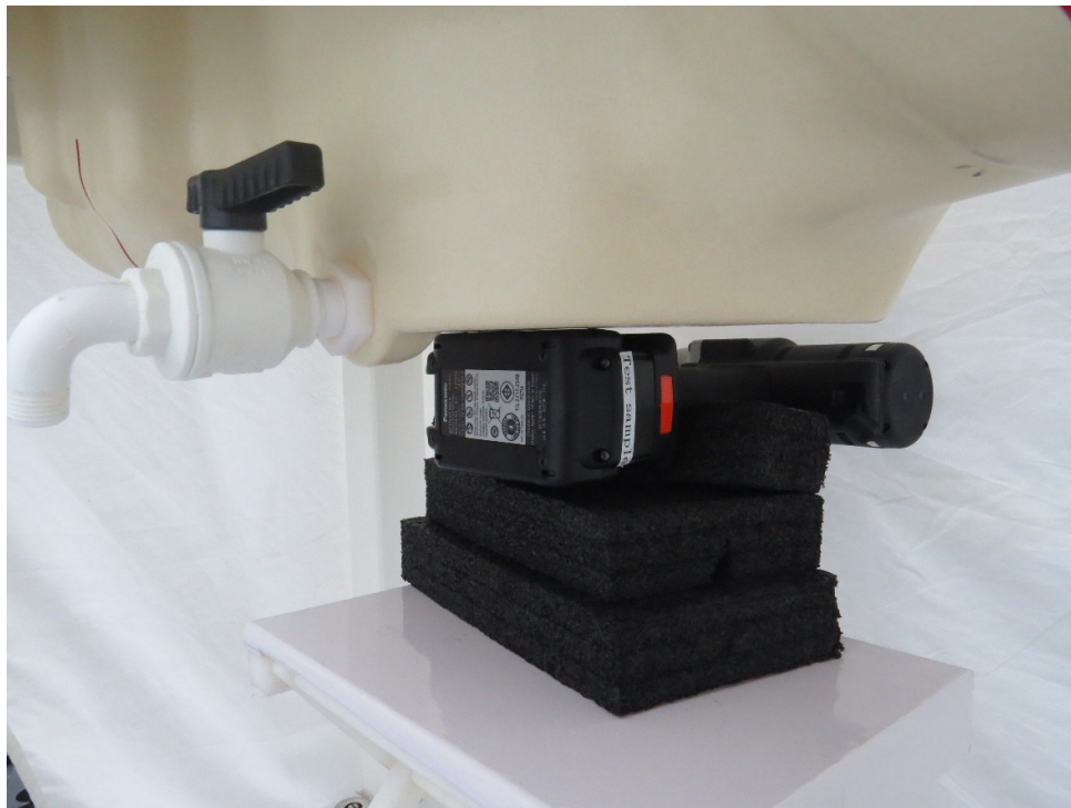
Picture 5: Right Edge, the distance from EUT to the bottom of the Phantom is 0mm
