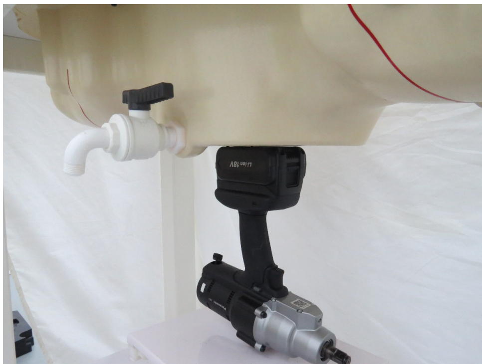
Picture 6: Bottom Edge, the distance from EUT to the bottom of the Phantom is 0mm
