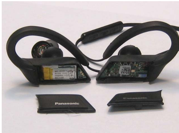
Left side (Battery and Thermistor board)
