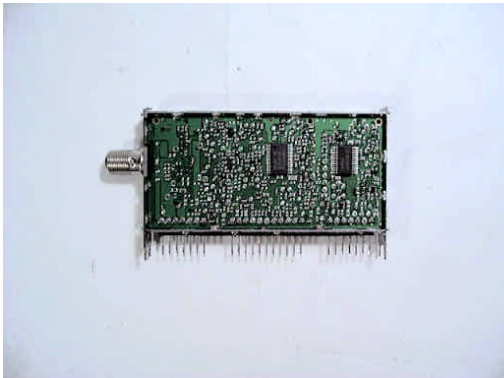
Tuner PCB (Bottom View)
