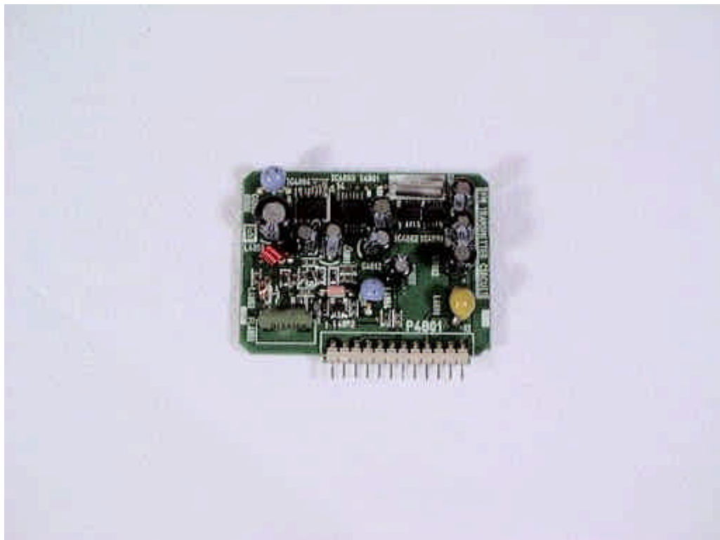
FM Transmitter PCB (Top View)
