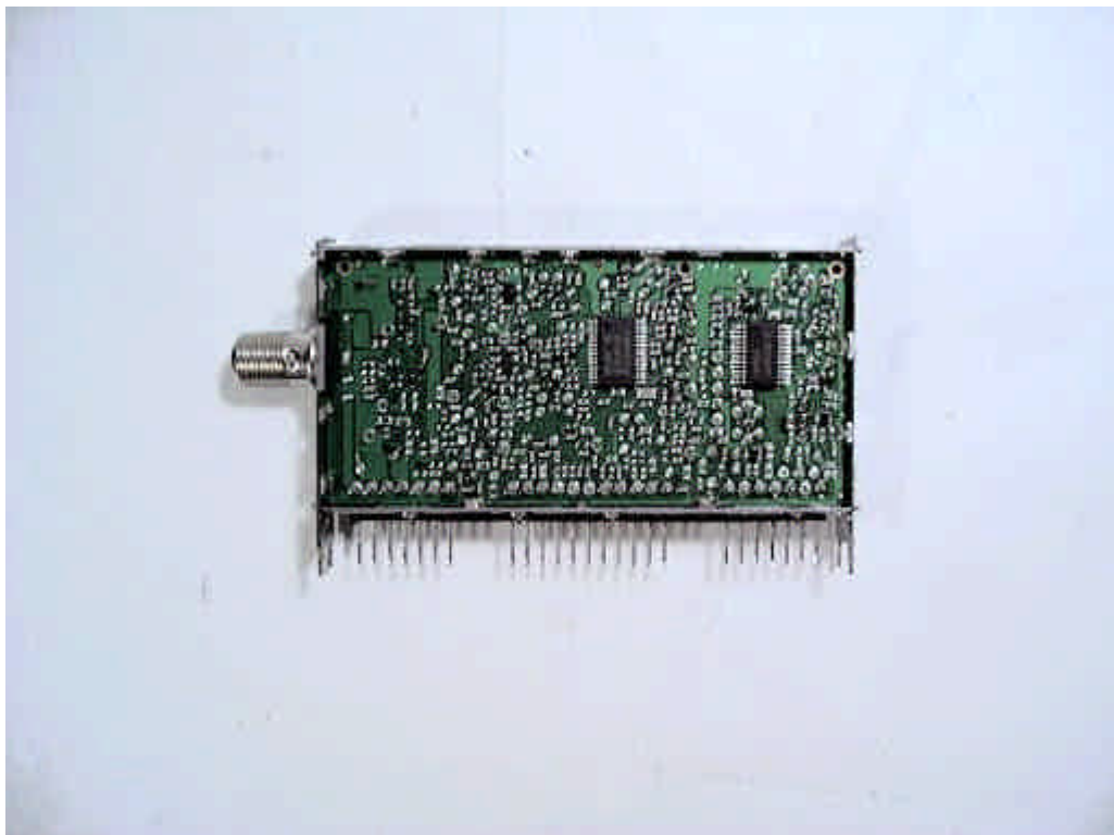
Tuner PCB (Bottom View)
