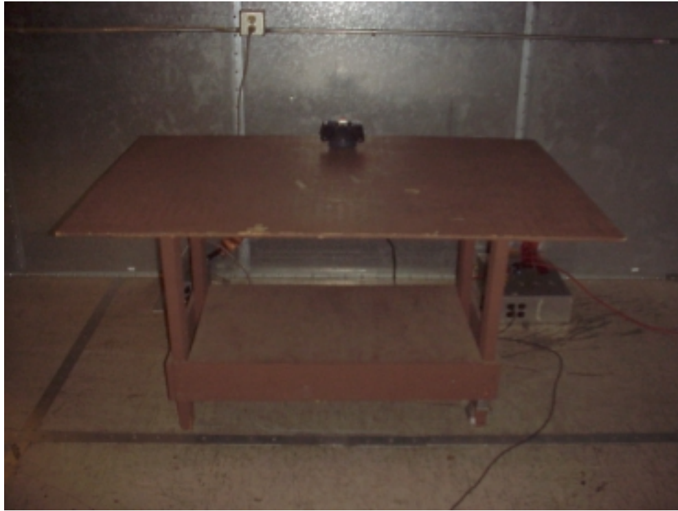
Photo: Conducted Emissions Charge Dock/Controller Unit (Front View)
