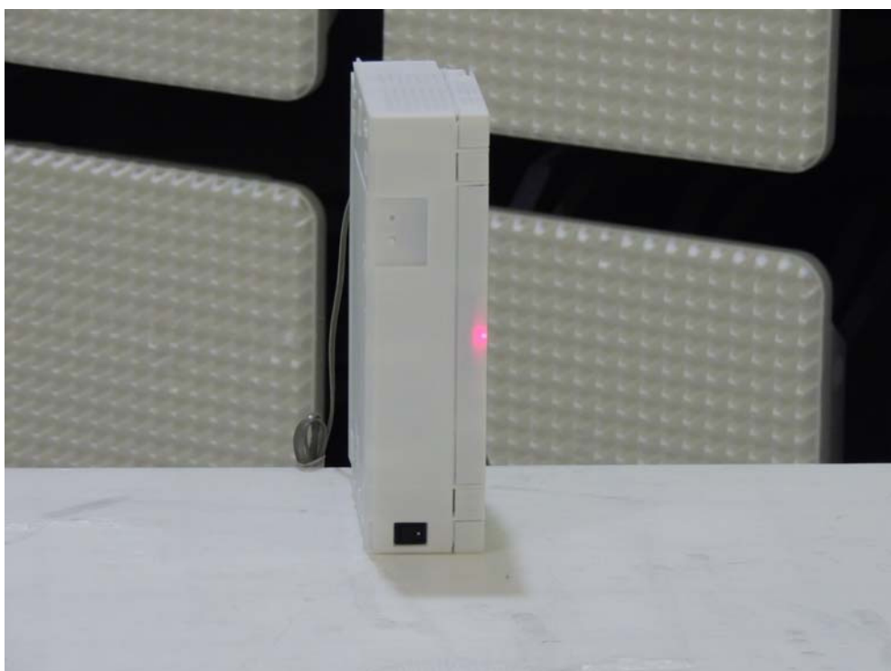
Photograph 7: Set-up for Radiated Emission, EUT Configuration Y-Axis
