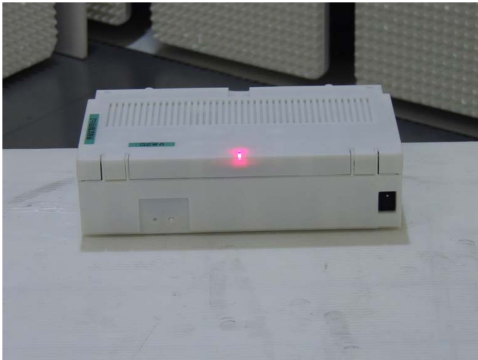
Photograph 6: Set-up for Radiated Emission, EUT Configuration X-Axis
