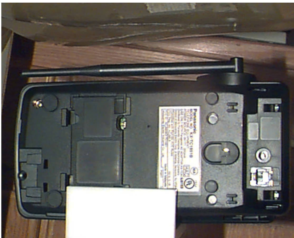
Figure 8. Test setup of EUT in normal operating position with the source of significant emissions (antenna) 2.0 cm below the phantom.
