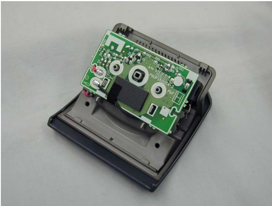
Internal view of battery charger
