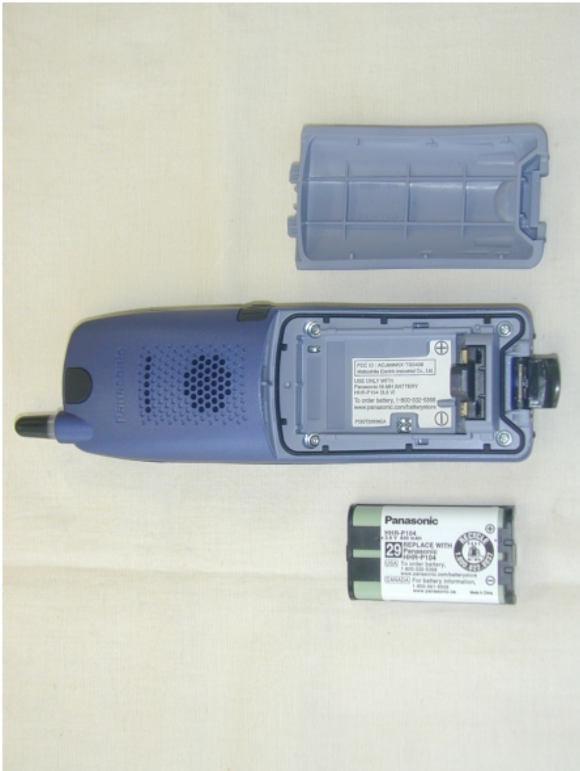
Battery Compartment Open
