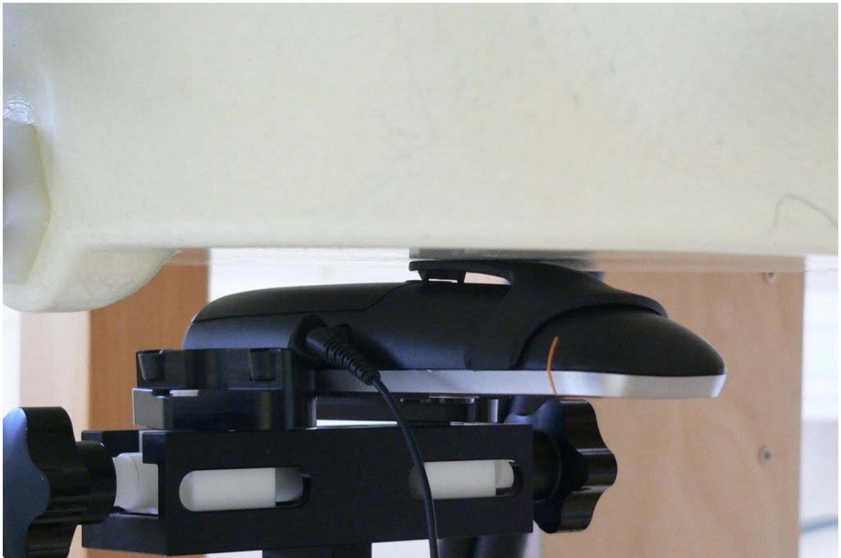
Fig. 21: Body worn configuration for KX-TGA680, position 2, display towards the ground, headset attached, 0 mm distance
