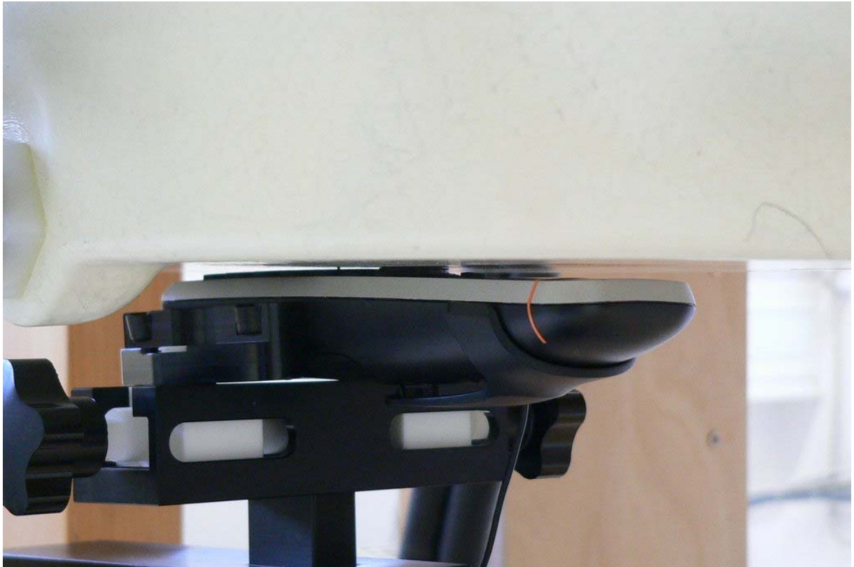
Fig. 20: Body worn configuration for KX-TGA680, position 1, display towards the phantom, headset attached, 0 mm distance
