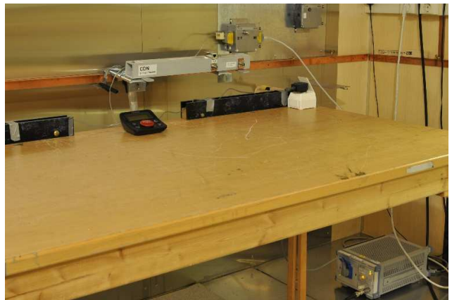
Conducted emission test
