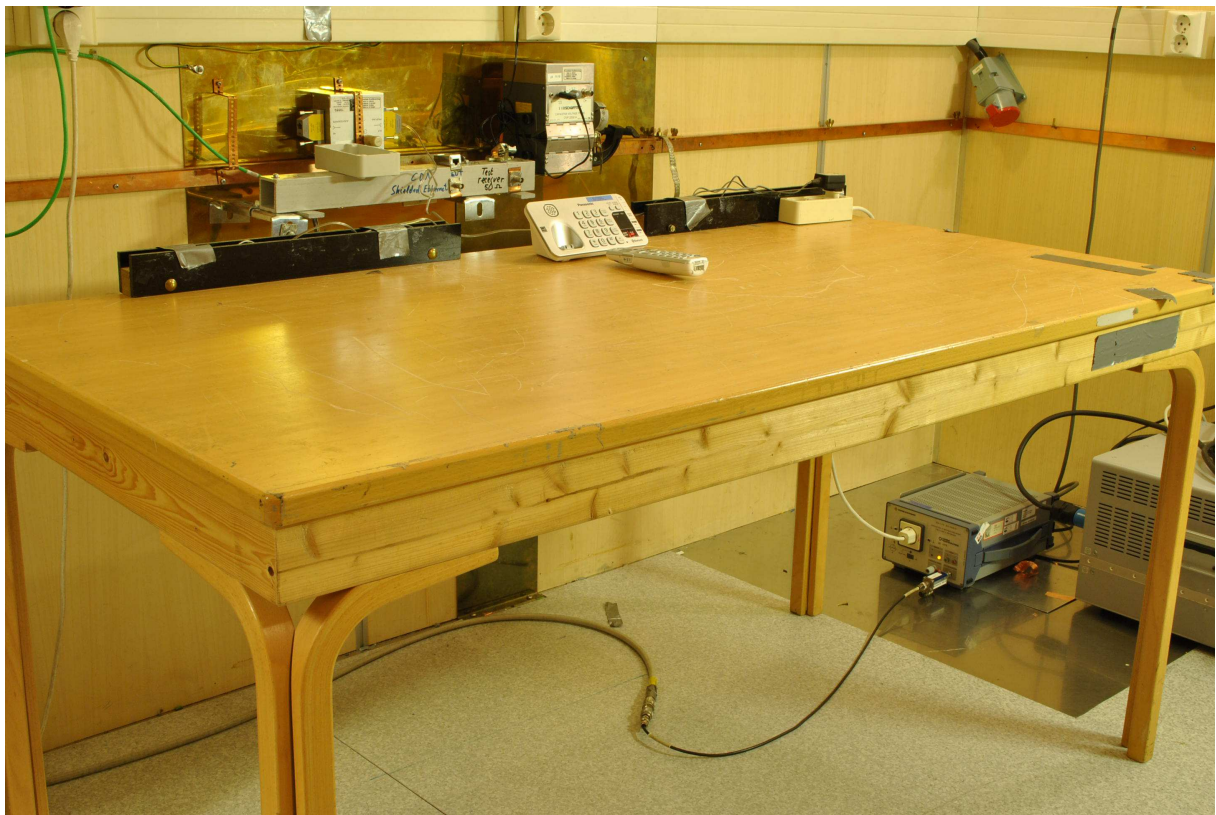
Power line Conducted Emissions Test
