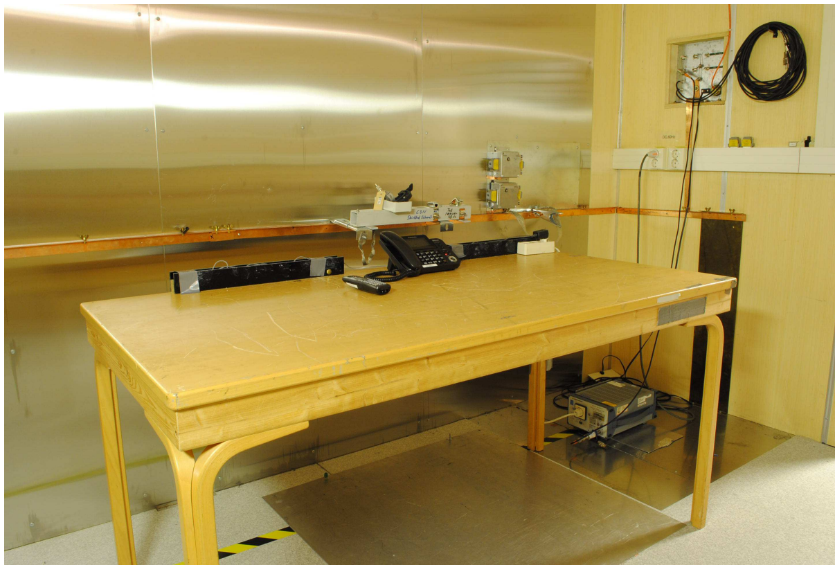
Power line Conducted Emissions Test
