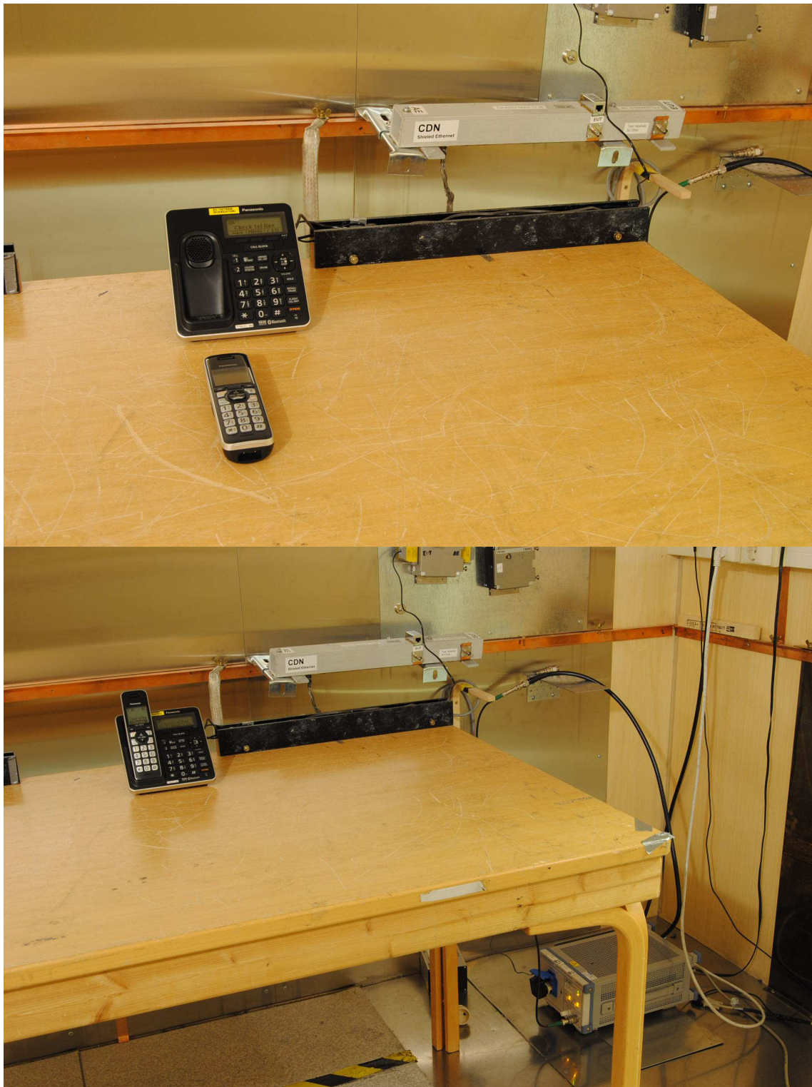
Power-Line Conducted Emissions Test
