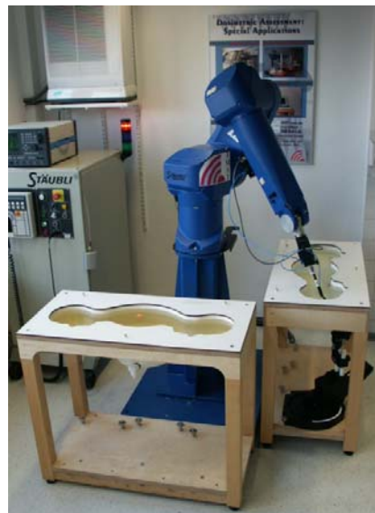
Fig. 8: The measurement set-up with two SAM phantoms containing tissue simulating liquid.
