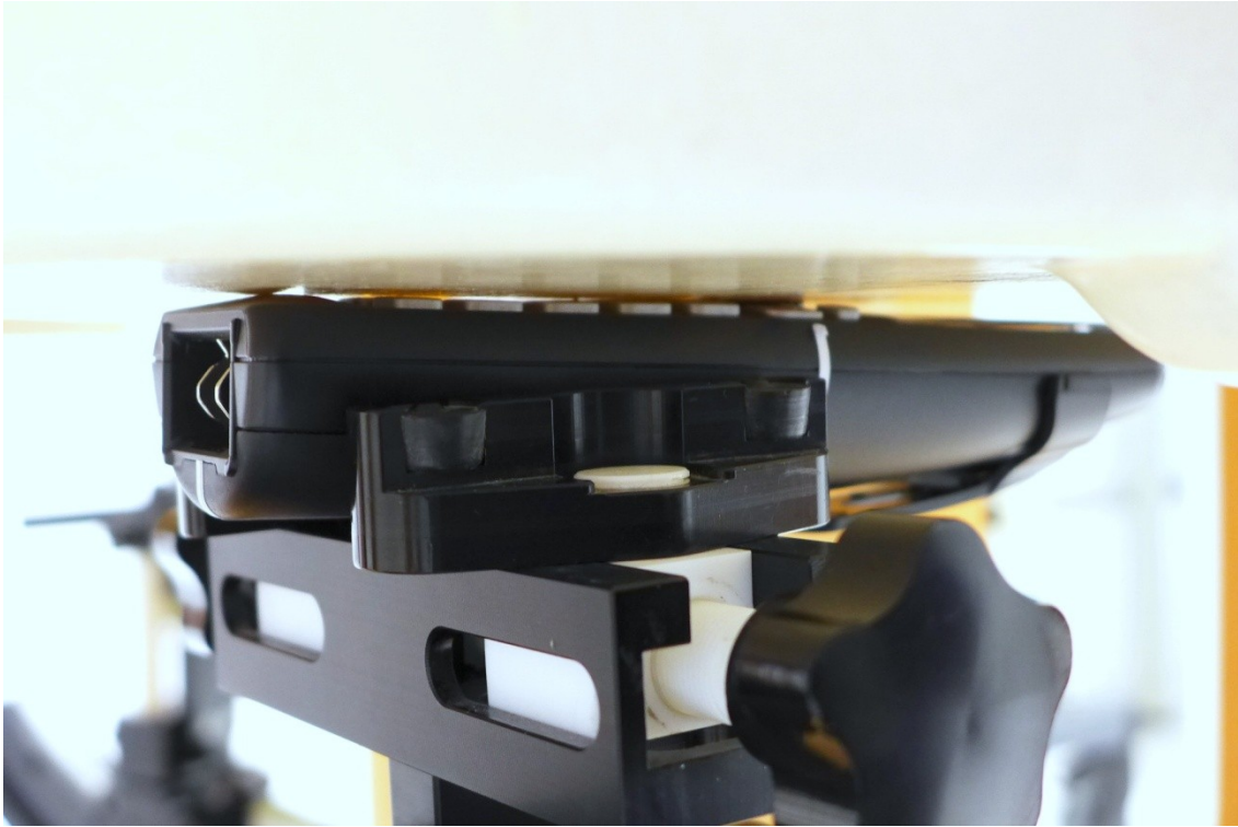
Pic. 7: Test position – front side, 0mm distance to phantom.
