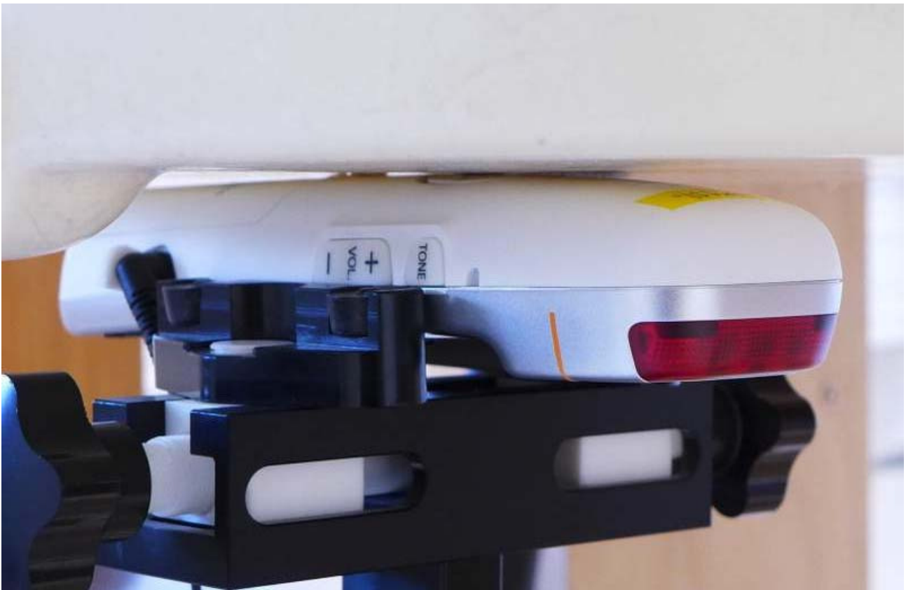
Fig. 20: Body worn configuration for KX-TGMA45, back of the device towards the phantom, headset attached, 0 mm distance.
