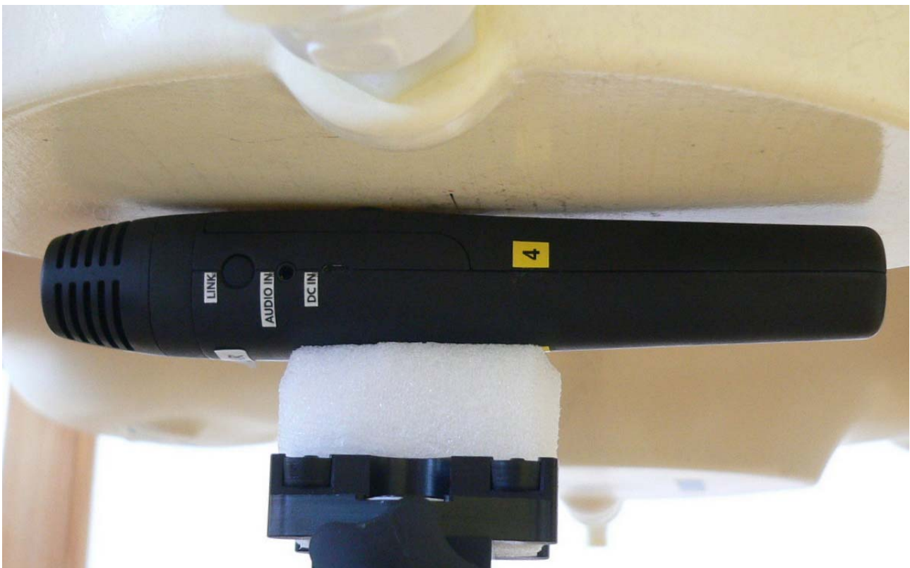
Fig. 11: Test position 2, back of the K-SHH14 towards the flat part of SAM phantom, 0 mm distance.
