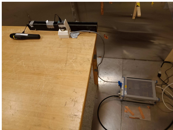
Power-Line Conducted Emissions
