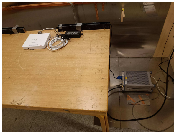
Power-Line Conducted Emissions
