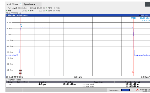
Peak Output Power, Upper Channel, HMA6RSP10 Cable
