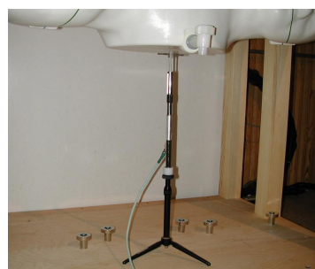
Figure 12.1 Dipole Validation Test Setup
