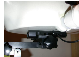
Figure 14.1 Body SAR Test Setup -- w/o Belt-clip --
