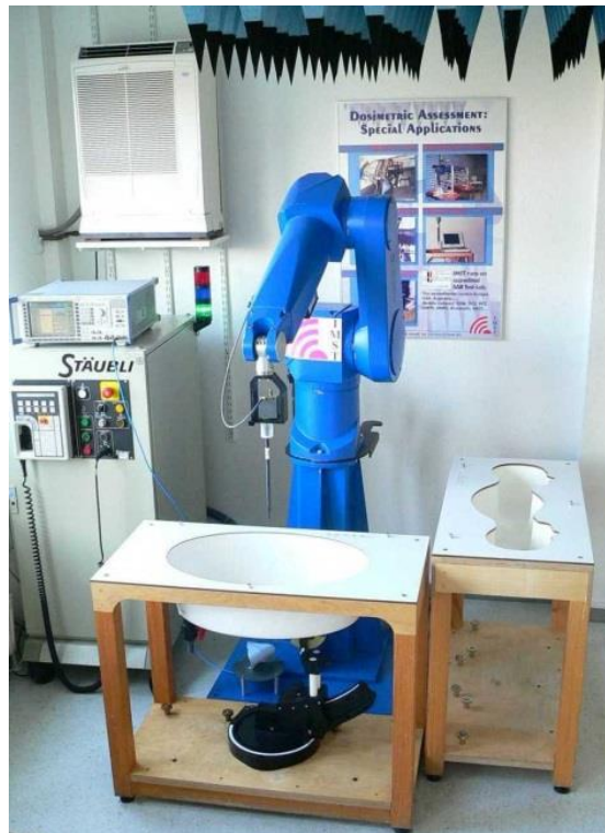
Fig. 3: The measurement set-up with a DASY system.
