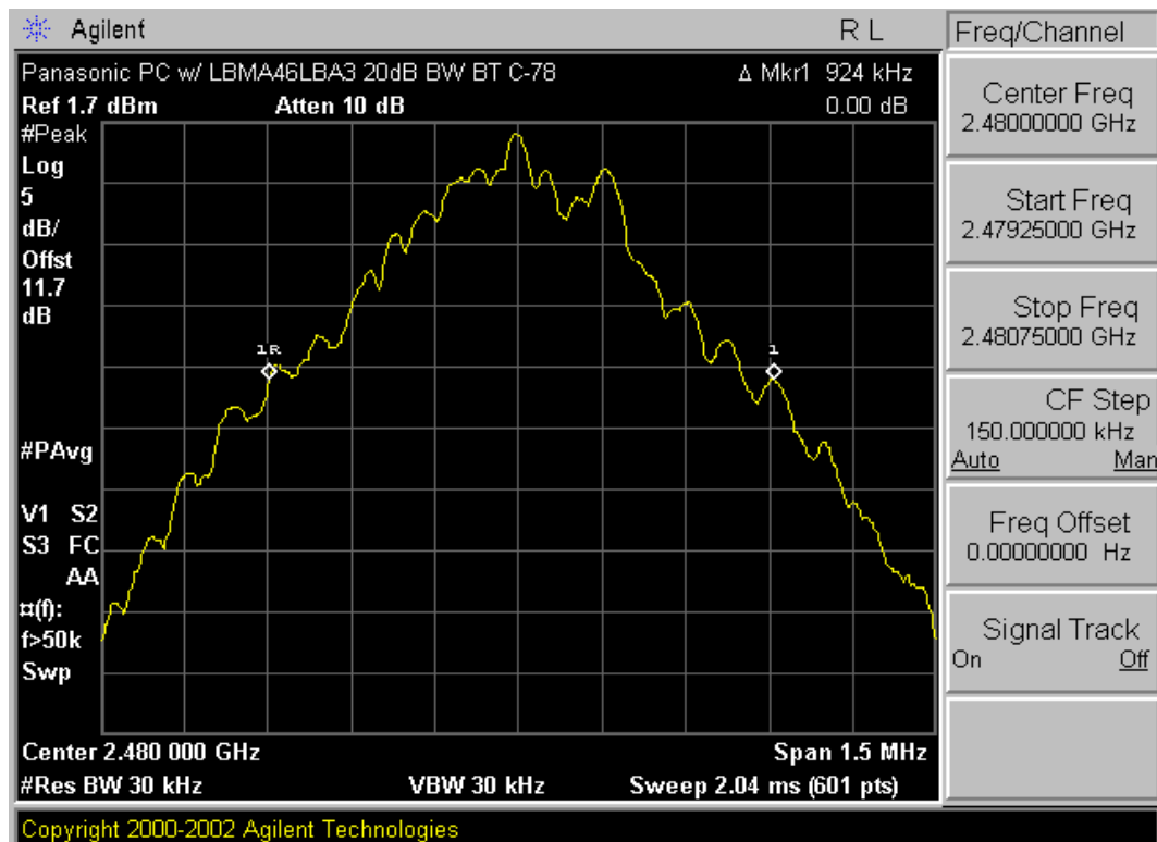
Plot 6-3. 20dB Bandwidth Plot (Bluetooth – Ch. 78)
