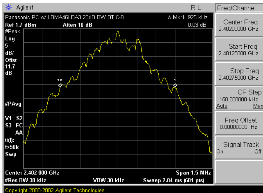
Plot 6-1. 20dB Bandwidth Plot (Bluetooth – Ch. 0)
