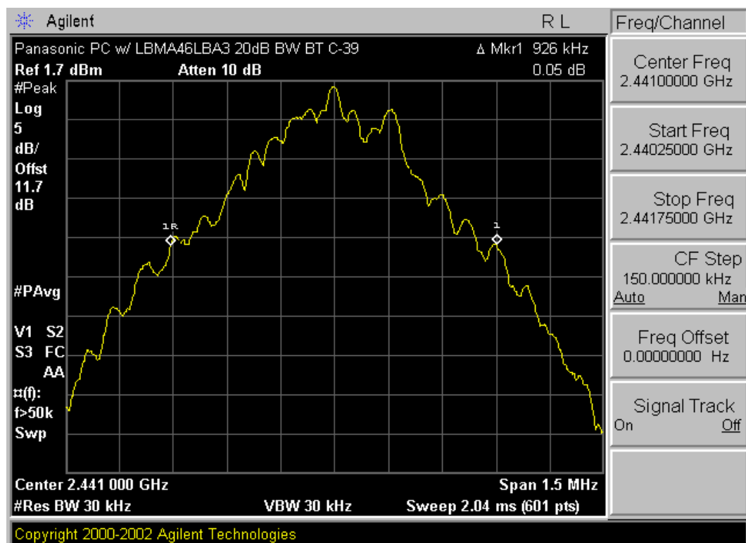
Plot 6-2. 20dB Bandwidth Plot (Bluetooth – Ch. 39)
