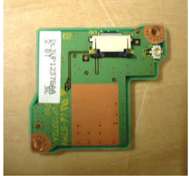
Bottom View of Bluetooth module with Daughter-Board
