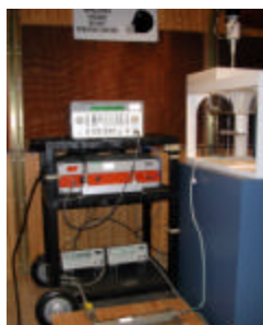
Figure A.0 Dipole Validation Test Setup
