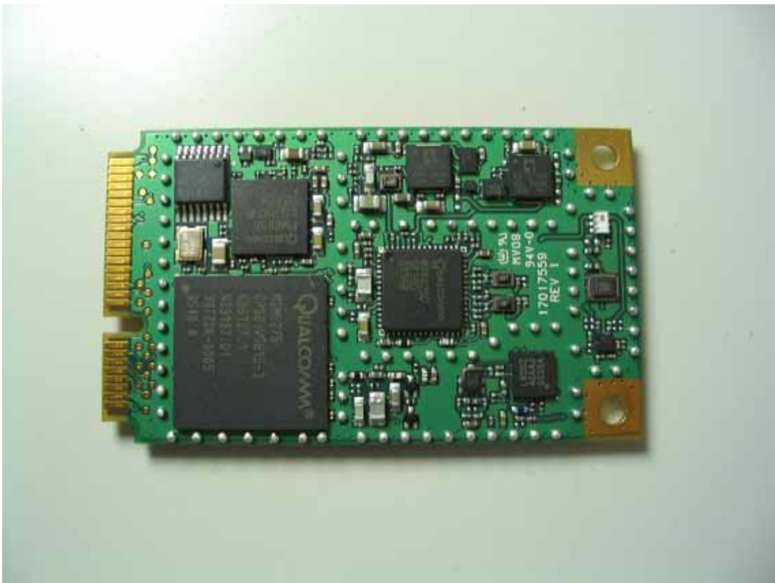
HSDPA Module Interior Bottom View
