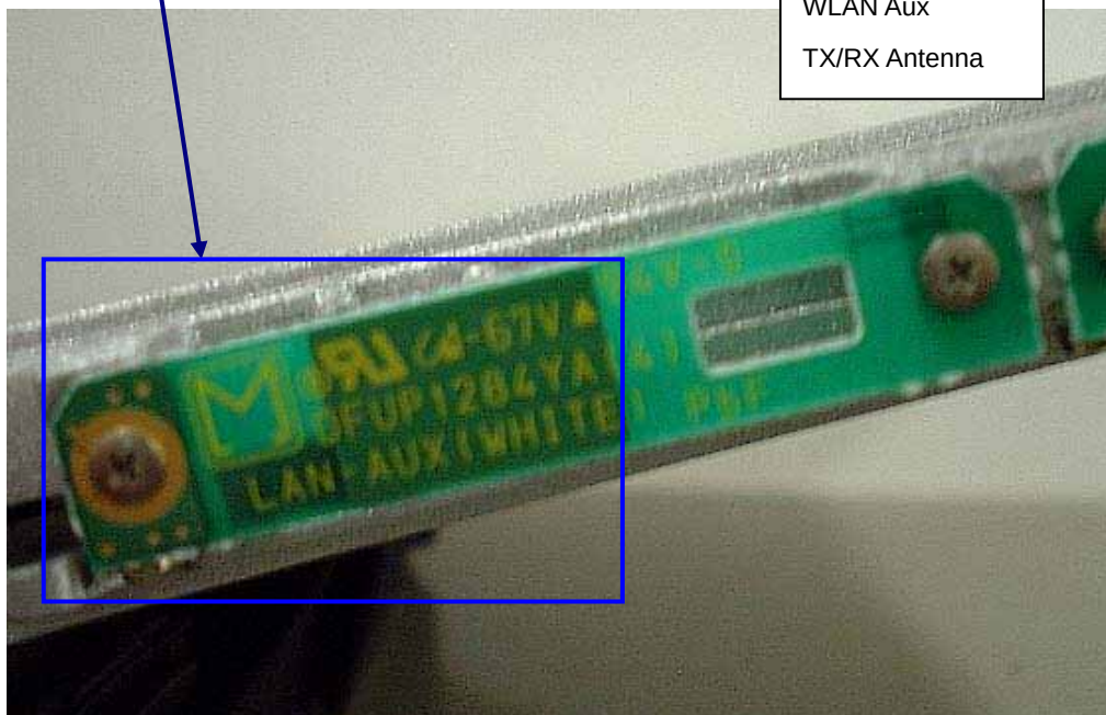
WLAN Aux TX/RX Antenna
