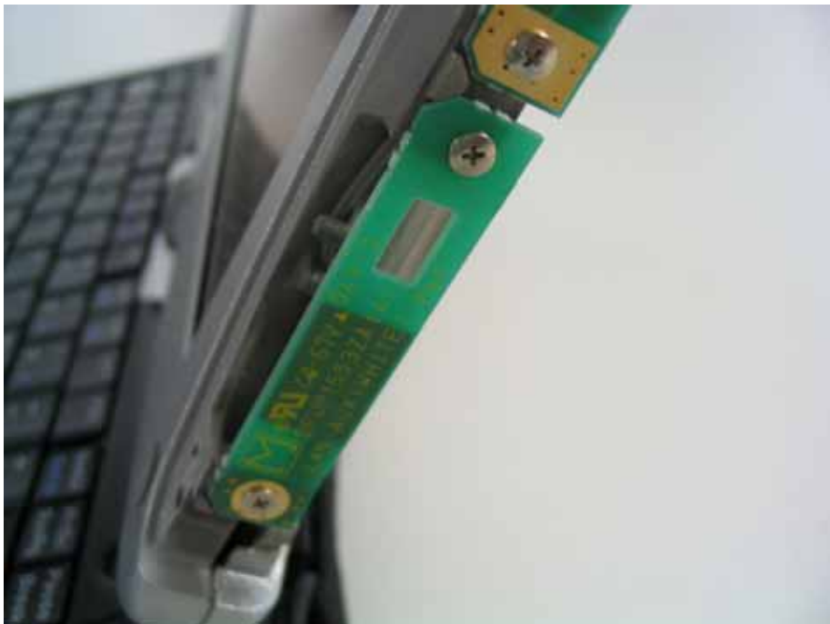
WLAN AUX TX/RX Antenna
