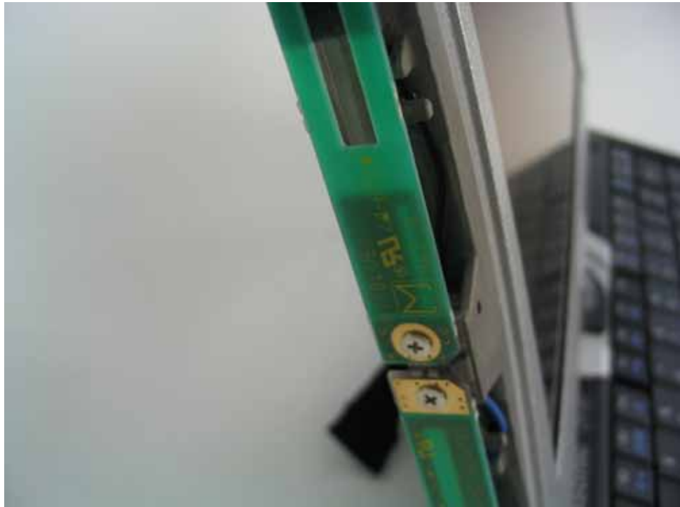
BlueTooth TX/RX Antenna
