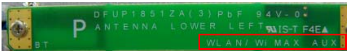
WLAN Aux TX/RX Antenna
