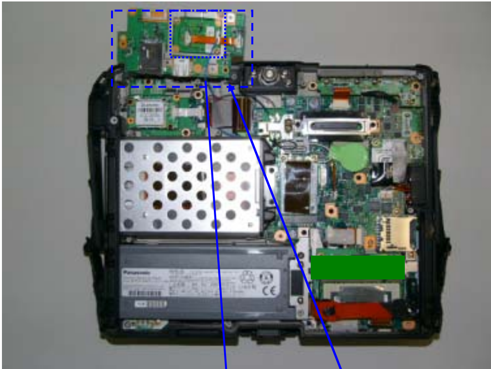
Reverse side of RF PWB
