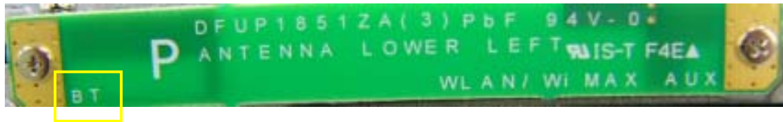
Bluetooth TX/RX Antenna
