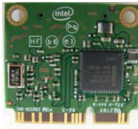
WLAN inside Bottom View
