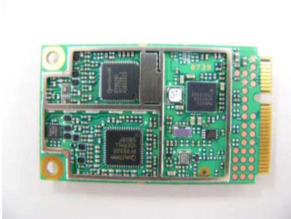
WWAN Inside Bottom View
