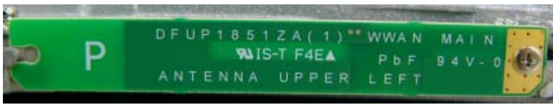
WWAN Main TX/RX Antenna
