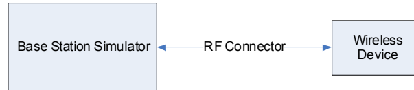
Figure 13-1 Power Measurement Setup
