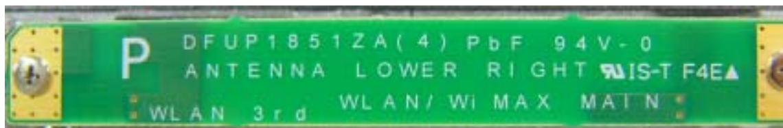
WLAN Main TX/RX Antenna
