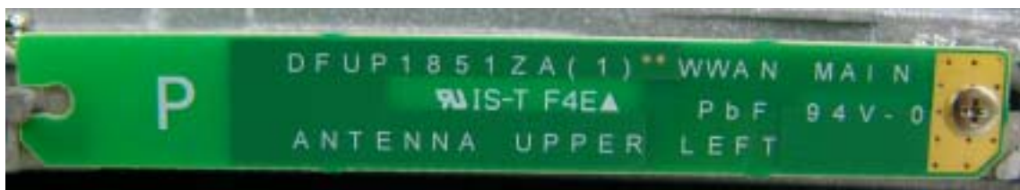
WWAN Main TX/RX Antenna
