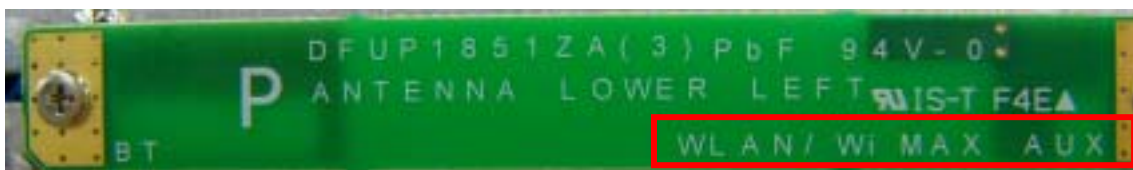
WLAN Aux TX/RX Antenna
