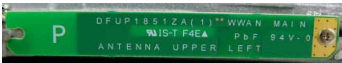
WWAN Main TX/RX Antenna
