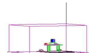
Figure 3-1. Shielded Enclosure Line-Conducted Test Facility
