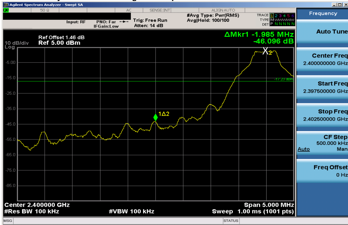
Plot 6-4. Band Edge Plot (Bluetooth – Ch. 0)
