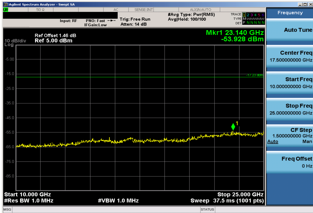
Plot 6-13. Conducted Spurious Plot (Bluetooth – Ch. 0)
