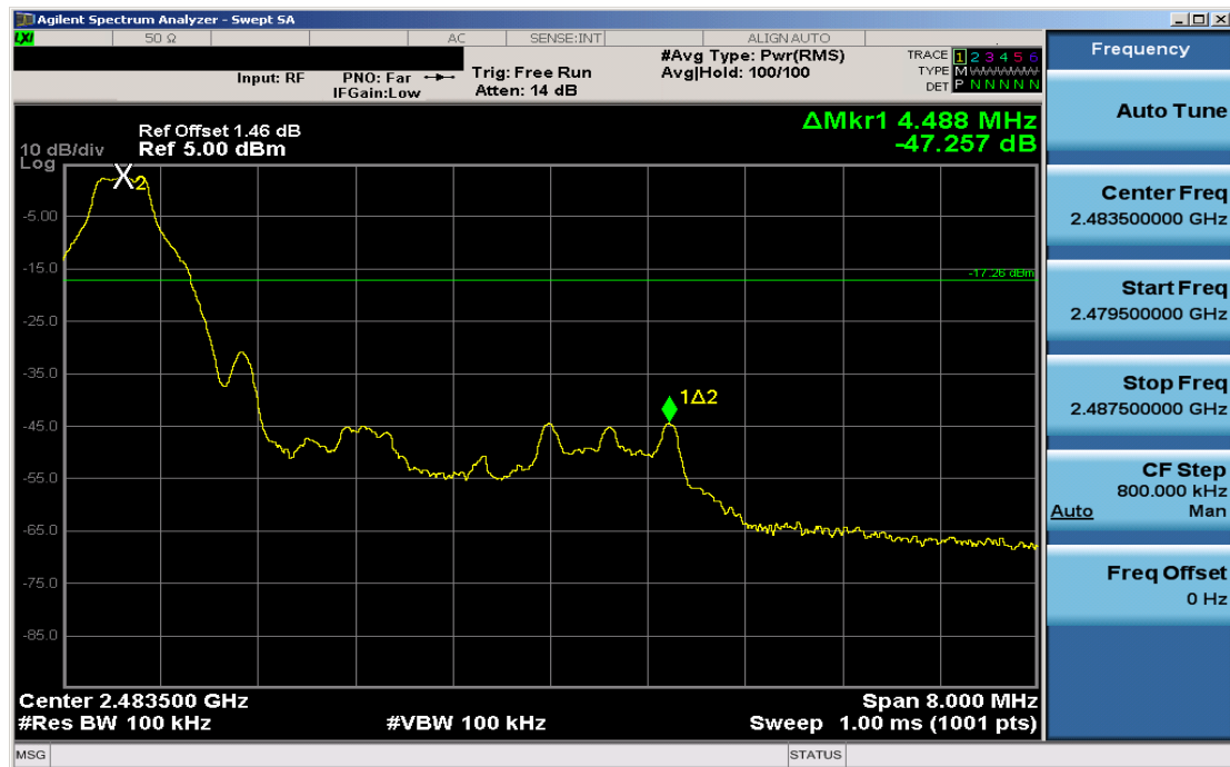
Plot 6-5. Band Edge Plot (Bluetooth – Ch. 78)
