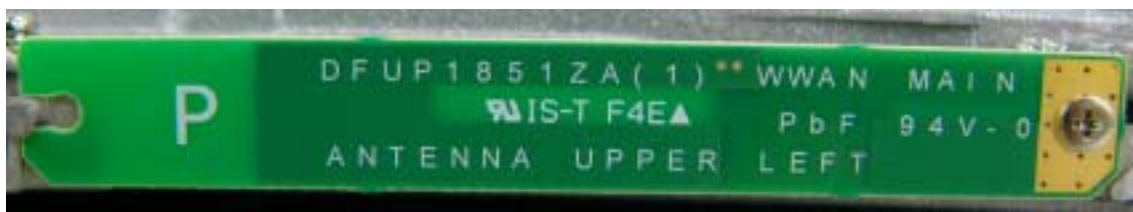
WWAN Main TX/RX Antenna
