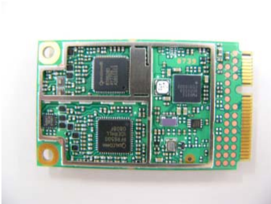
WWAN Inside Bottom View
