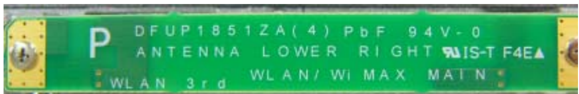
WLAN Main TX/RX Antenna
