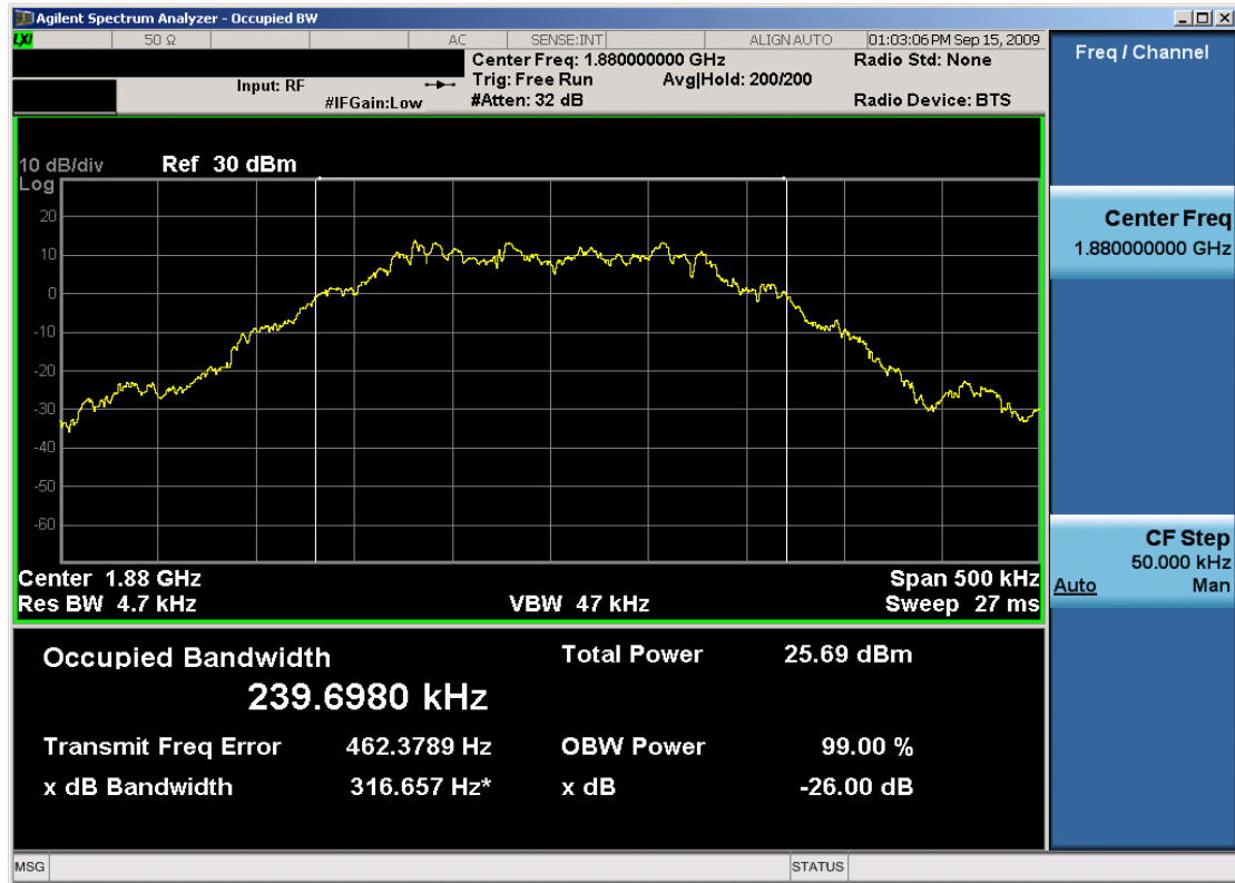
Plot 7-21. Occupied Bandwidth Plot (EDGE1900 Mode – Ch. 661)
