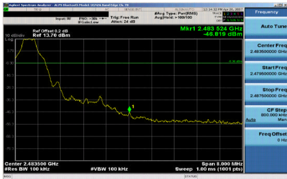
Plot 6-5. Band Edge Plot (Bluetooth – Ch. 78)
