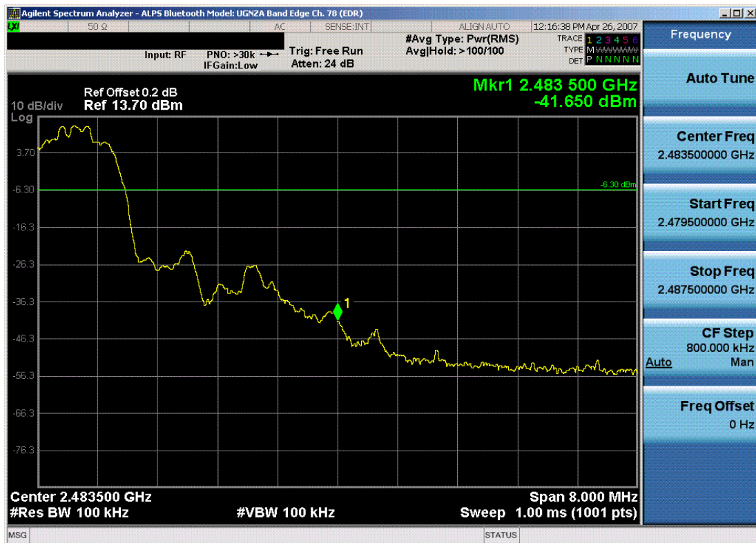
Plot 6-7. Band Edge Plot (Bluetooth 2.0 with Enhanced Data Rates – Ch. 78)
