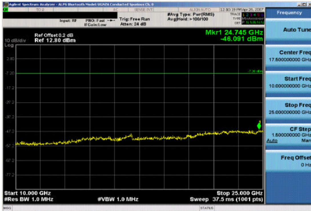
Plot 6-13. Conducted Spurious Plot (Bluetooth – Ch. 0)
