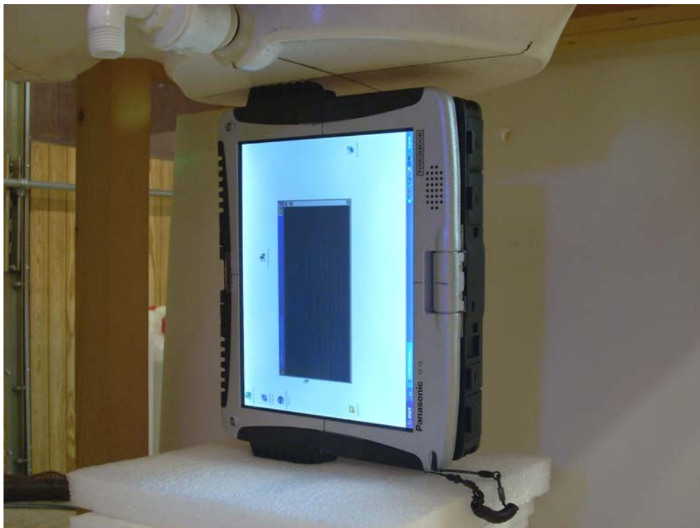
Figure 19-4 SAR Test Setup Photo 4 (Tablet Right)
