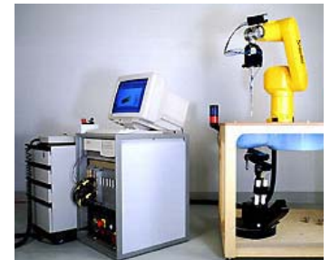
Fig. 1 SAR Test Setup
