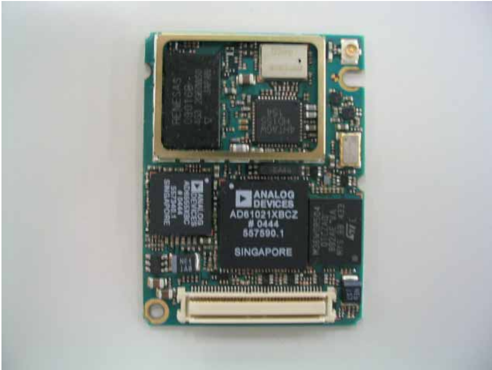
MC75 Module Interior Top View
